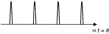
Fig. 4.20. Equidistant pulses seen as a function of phase \phi
